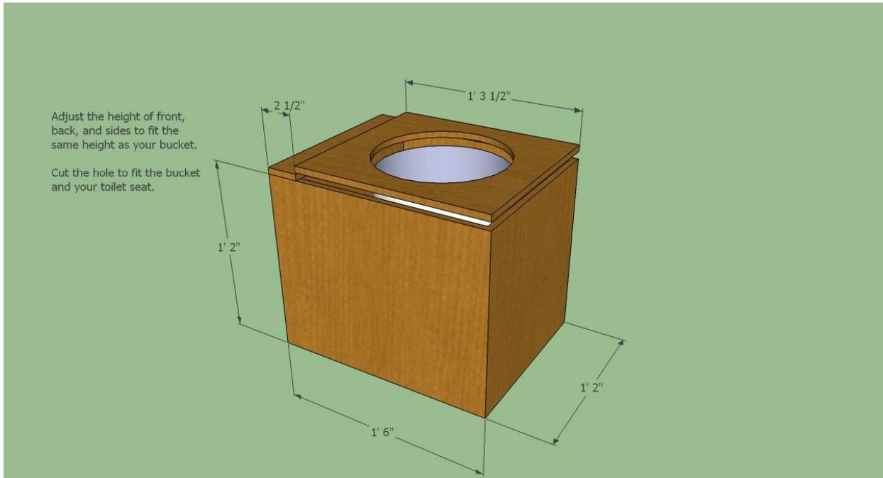
This was a simple composting toilet built from scrap 3/8" plywood. The seat and 5 gallon bucket that I ended up using was only \$9.27 after taxes. This project took 2 hours to put together, sand and lacquer. Overall this was a quick project, and if you have to buy a set of hinges, can of lacquer, and the plywood and nails, you can build this for less than US\$20.00. This can support my body weight of 212 pounds.
