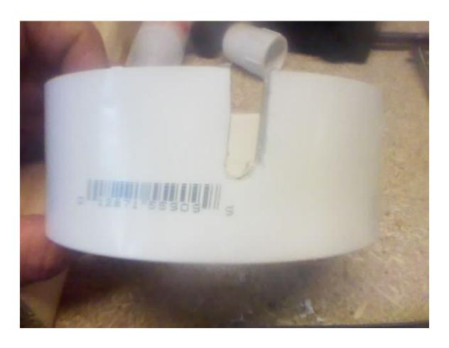
Drill a  $\frac{1}{4}$ " hole centered on the side of the coupler. Cut a  $\frac{1}{4}$ " slot to the hole. This will be for the power cord that is attached to the fountain pump.
