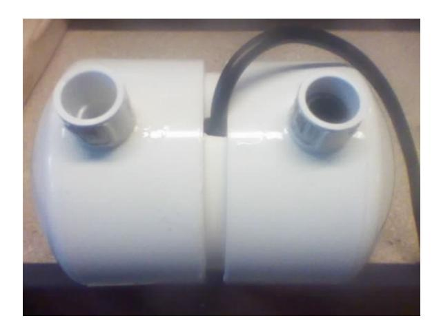
Slop up the inside of the PVC end cap with PVC Cement as well as the coupler that now holds the other half with the pump. Slip the end cap over the coupler and turn slightly back and forth to bond the PVC Cement and the two PVC pieces together.
