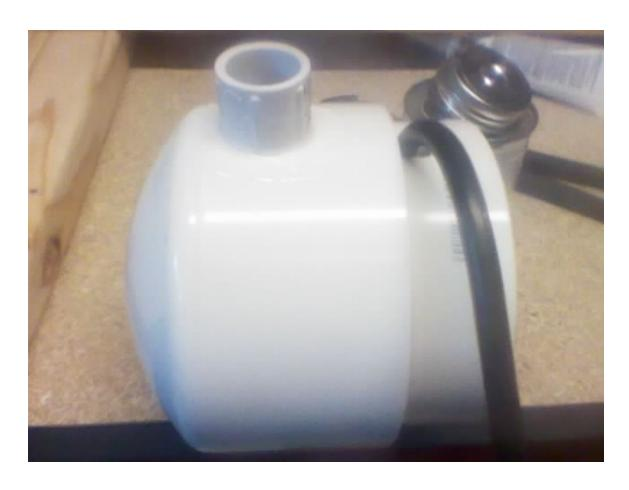
Apply PVC Cement to the outside of the fountain pump outlet. Apply PVC Cement to the threads of the male coupler. Thread in the <sup>3</sup>/<sub>4</sub>" male coupler into the hole over the fountain pump outlet. This will join the fountain pump to the coupler as well as join the "outlet" to the housing so that our pump is now hard mounted.
