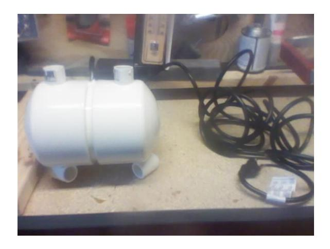
The end result is a US\$61.05 in-line pump that will connect to the existing lines. This will have a down force of 5 gallons per minute which will be more than enough to provide water to the 1.2 GPM toilet and the 1.8GPM shower. I will still have 2GPM to spare to provide plenty of water to my kitchen sink. This all comes in at a whopping 8.5 watts of electricity. I can't complain.
