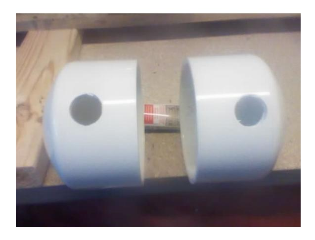
Drill 1" holes towards the end of both 4" end caps. These are what will become the inlet and the outlets of our in-line pump.
