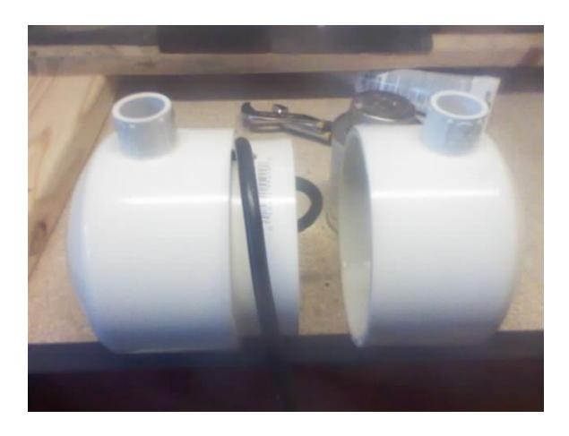
Apply PVC Cement to the threads of the male coupler. Thread in the  $\frac{3}{4}$ " male coupler the hole on the inlet. This will provide a hard mounted inlet.
