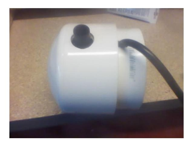
Slop up the inside of the PVC end cap with PVC Cement as well as the coupler that now holds the fountain pump. Slip the end cap over the fountain pump and turn slightly back and forth to bond the PVC Cement and the two PVC pieces together.
