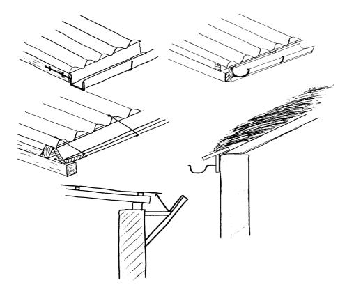
Figure 5: a variety of guttering types showing possible fixings
