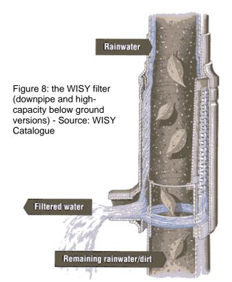
rudimentary. A German company, WISY, have developed an ingenious filter which fits into a vertical downpipe and acts as both filter and first-flush system. The filter, shown in Figure 8, cleverly takes in water through a very fine (~0.20mm) mesh while allowing silt and debris to continue down the pipe. The efficiency of the filter is over 90%. This filter is commonly used in European systems.
