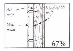
Sheet metal shields or those backed with sheet metal give greater reductions in clearance because of their ability to conduct heat rapidly across their surface, reducing the intensity of hot spots.
