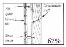
Sheet metal shields with 21 mm ('/8") air space behind give a 67% reduction in the minimum clearance. Brick or tile shields backed with sheet metal also give a 67% reduction in clearance.
