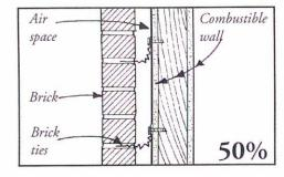
Brick shields without steel backing (above) give only a 50% reduction in clearance. Shields constructed of tile on non-combustible board (below) also give a 50% clearance reduction.
